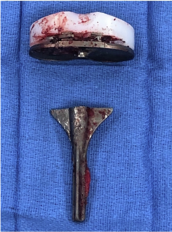
Figure 2. Catastrophic failure of the component. Intraoperative photograph demonstrating fracture and catastrophic failure of the tibial component. The tibial baseplate and well-fixed polyethylene were completely dissociated from the stem portion of the tibial component.
