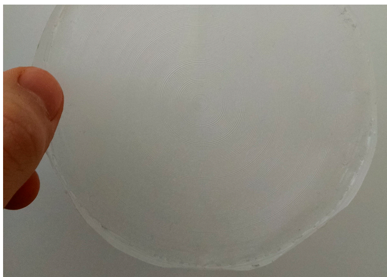
Figure 5. Thin transparent film of functionalized PE-HEMA obtained via solution casting.
