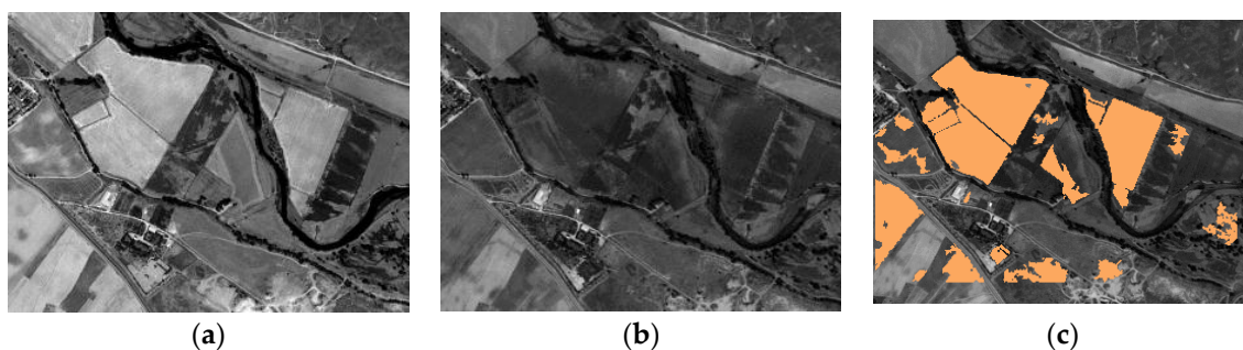
Figure 16. DS1 subset example for object based analysis: (a) 2005 SPOT-PAN image subset; (b) 2008 SPOT-PAN image subset; (c) Test objects.
