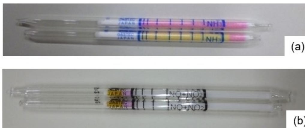
Figure 6. Photographs of tubes used to detect (a) \text{NH}_3 and (b) \text{NO}_x before (upper tube) and after (lower tube) injection of gas in the reactor. The \text{NH}_3 detecting tube was pink before use and changed to yellow when \text{NH}_3 was detected. The \text{NO}_x detecting tube was white before use and would have changed to orange-yellow if \text{NO}_x had been detected.
