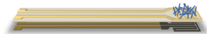
Figure 1. Al 2 O 3 substrate with \beta -Ga 2 O 3 nanowires grown on Au interdigitated electrodes. Pt meander-type heater was screen printed on the bottom side of the substrate.
