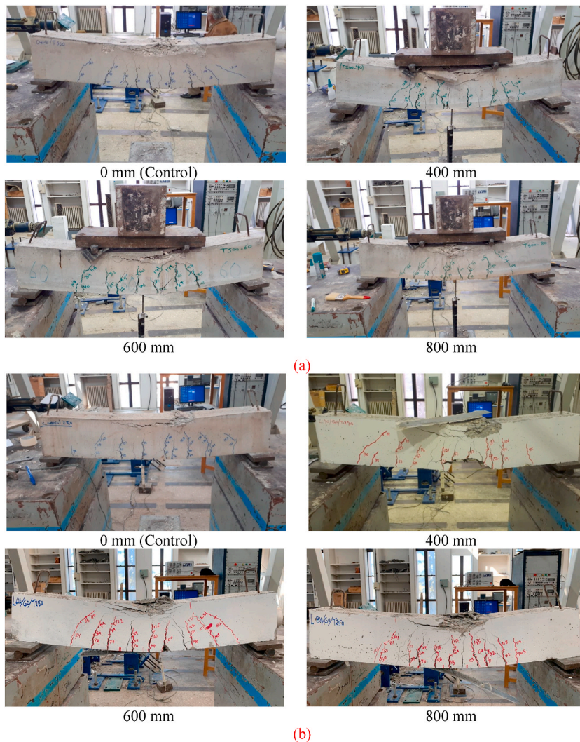
Fig. 11. The impact of strengthening technique on the mode of failure of (a) Internal strengthening, and (b) External strengthening.
