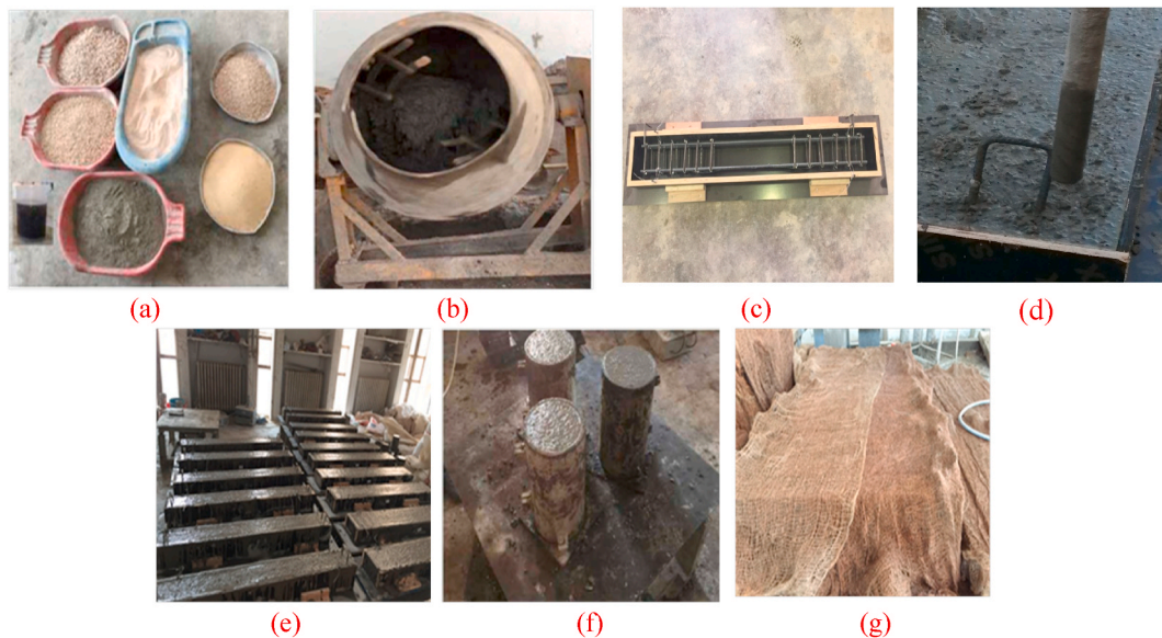
Fig. 4. Preparing of reinforced concrete beams (a) Mixture ingredients preparation, (b) Tilting drum mixer, (c) Wooden mold, (d) Vibrator compacting, (e) Concrete casting, (f) Cylinders casting, and (g) Beams curing for 28 days.
