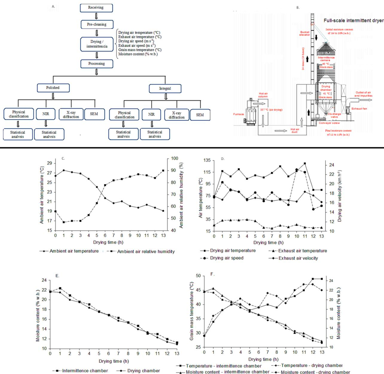
**Fig. 1.** Flowchart demonstrating the rice evaluation process (A), full-scale intermittent dryer (B), and parameters for monitoring the intermittent drying of rice paddy, ambient air temperature and relative humidity (C), drying and exhaust air temperature and velocity (D), drying curve (E), grain mass temperature and moisture content at drying (F).
