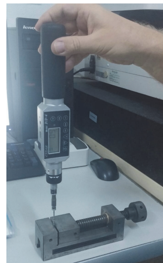
FIGURE 3: Measurement of loosening torque using a torque tester.
