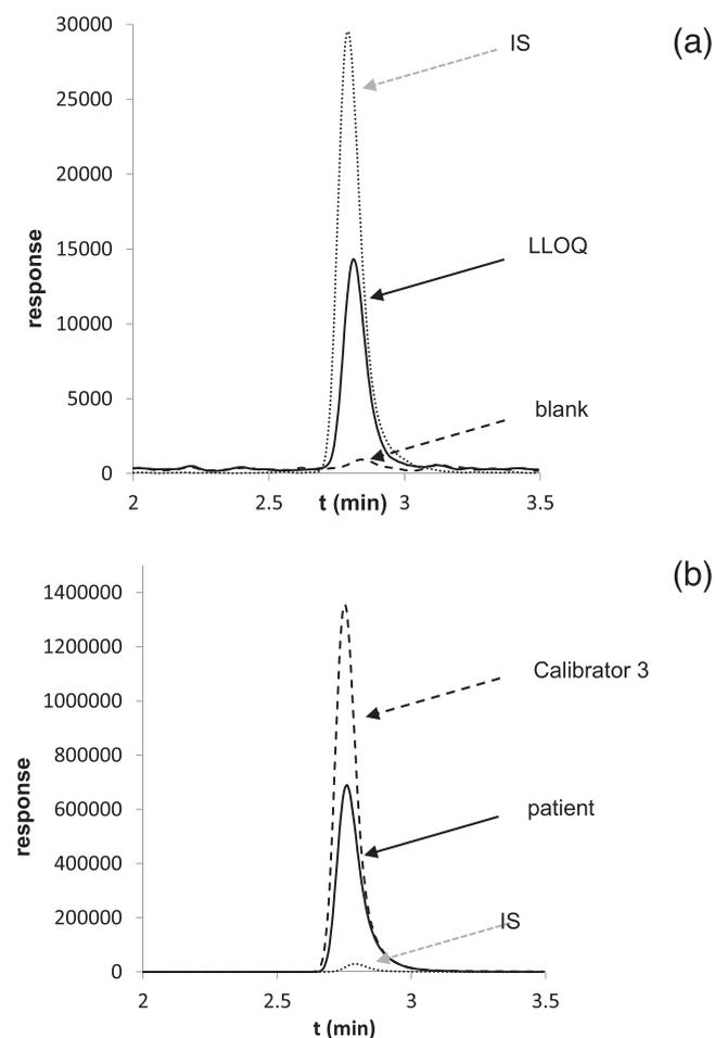
**FIGURE 2** MRM (multiple reaction monitoring) chromatograms of an (a) LLOQ (lower limit of quantification) sample, blank, and IS (internal standard) and (b) calibrator 3, study sample, and IS
