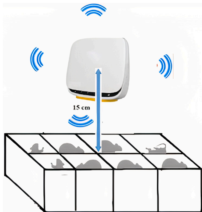
Fig. 1. The rats were in a plastic cage 55 \times 32 \times 20 cm, but not free to move with restrictions in the cage during exposure. Wi-Fi emitter emitted a continuous wave for 2, 24 h, 72 h, frequency 2.450 GHz frequency band, power density = 4.2 \text{ nW/m}^2 at 15 cm. The cage was surrounded with electromagnetic absorber material backed by metal to isolate outdoor electromagnetic fields from the test setup during exposure.
