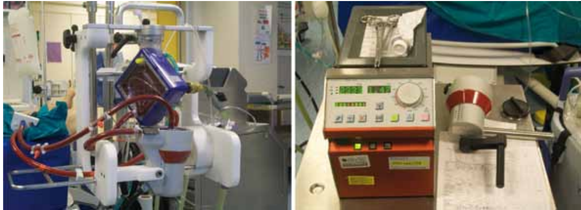
Figure 1 - ECMO circuit with membrane oxygenator and centrifugal pump mounted on a specially designed multifunctional holder Steering and control unit including battery pack.
