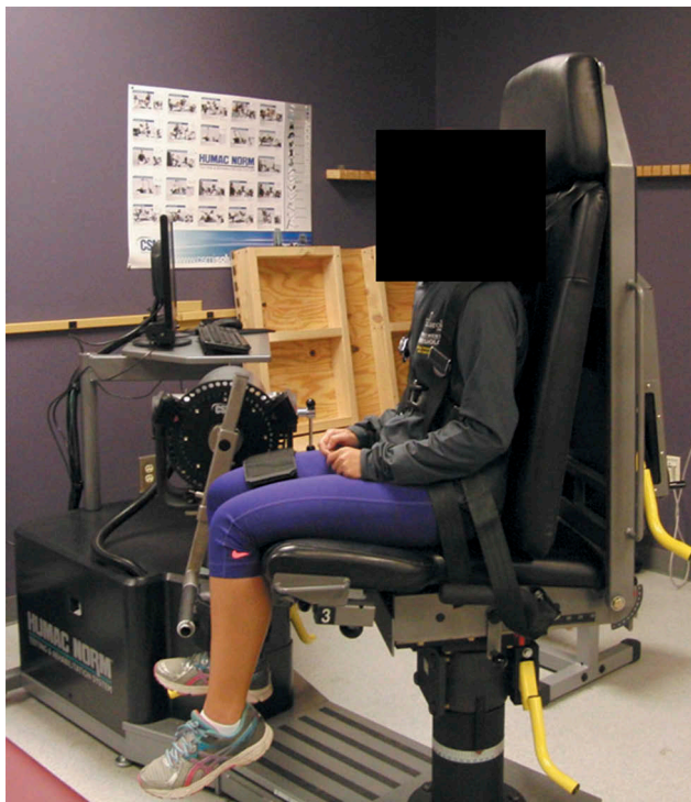
Figure 1. Experimental setup for isometric knee extensor strength testing.
