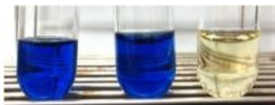
Figure 5. Decolorization of indigo carmine by the IOX/iodide system. The reaction mixture contained 10 mU mL -1 of IOX, 0.3 mM indigo carmine, 0.1 mM iodide, and 20 mM sodium acetate buffer (pH 5.5). The reaction time was 5 h. The left and middle tubes are negative controls in which IOX and iodide were omitted from the reaction mixture, respectively.
