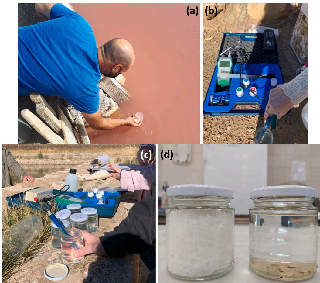
Fig. 1. Panel a, sampling in the field; Panel b and c, pH and salinity measurement; Panel d, samples.
