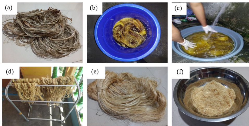
Figure 1. Kenaf fibre preparation process: (a) kenaf fibres post-extraction, (b) treatment in alkaline immersion, (c) pH neutralisation with an acetic acid solution and rinsing, (d) drying, and (e) cutting to short kenaf fibres.
