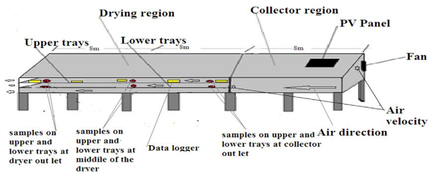
Figure 2. Arrangement of the instruments in the twin layer solar tunnel dryer.
