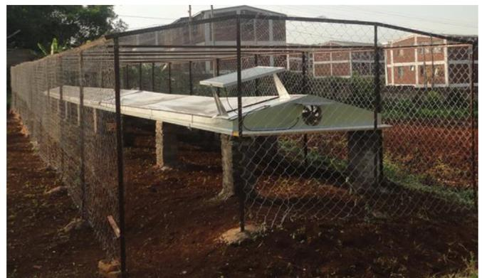
Figure 1. Twin layer solar tunnel dryer Photo.
