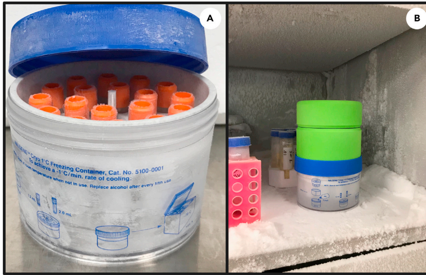
Figure 6. Cooling of E. gracilis cells in Mr. Frosty placed in a -80^{\circ}\text{C} freezer
