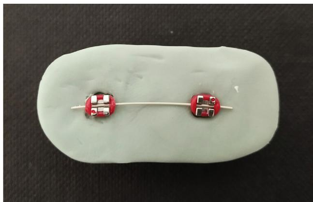
**Fig. 2** Archwire specimen ligated on brackets embedded in an acrylic block.
