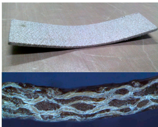
Figure 6. Typical flexural failure of flax/PP composites.
