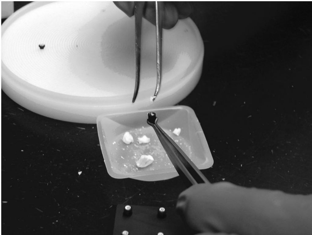
FIG. 6. Loading freeze-dried organisms into Phobos LIFE sample tube.
