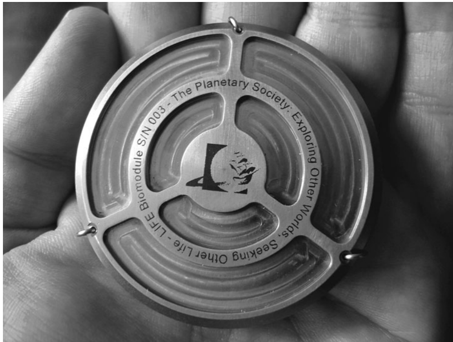
FIG. 1. Sealed Phobos LIFE biomodule. Hand for scale.
