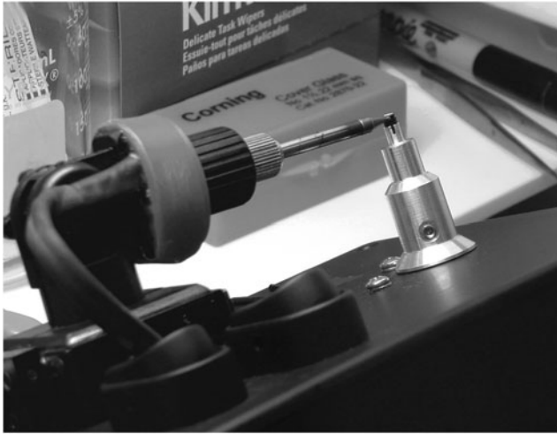
FIG. 3. Heat sealing a sample tube inside argon-filled glove box.
