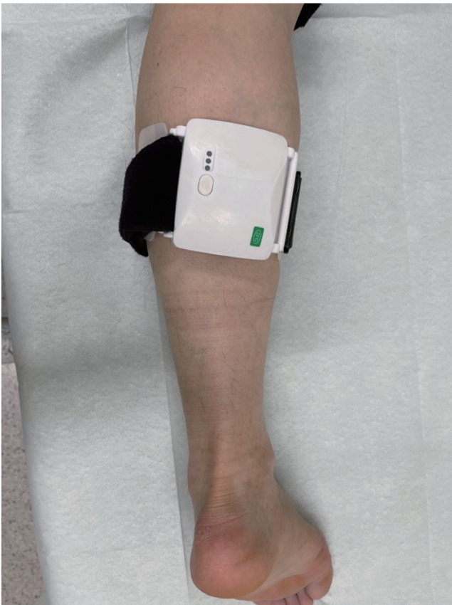
Fig. 1. Photograph of the spinning permanent magnet (SPM) device attached to the patient's lower leg. The device is compact and lightweight, measuring 7.5 \times 6.3 \times 2.5 cm and weighing 165 g. It can easily be attached to limbs using the Velcro strap.
