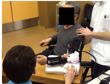
Fig. 1. HAL-SJ intervention to the participant’s elbow on the paralytic side.
