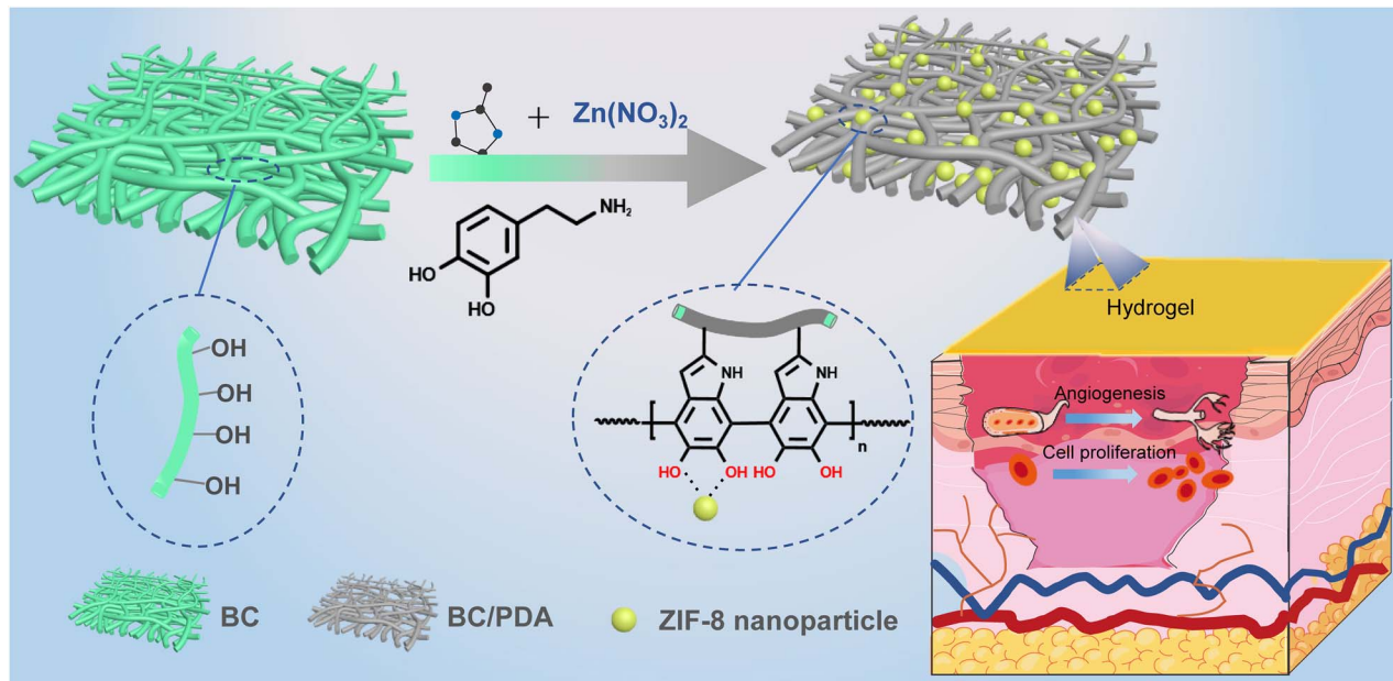
Figure 1. Preparation of BC/PDA/ZIF8 hydrogels. BC bacterial Cellulose, PDA polydopamine, ZIF8 zeolitic imidazolate framework 8
