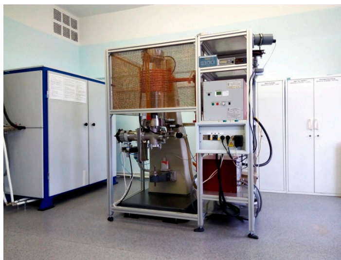
Figure 2. Technological setup for the growth of graphene on the SiC surface.
