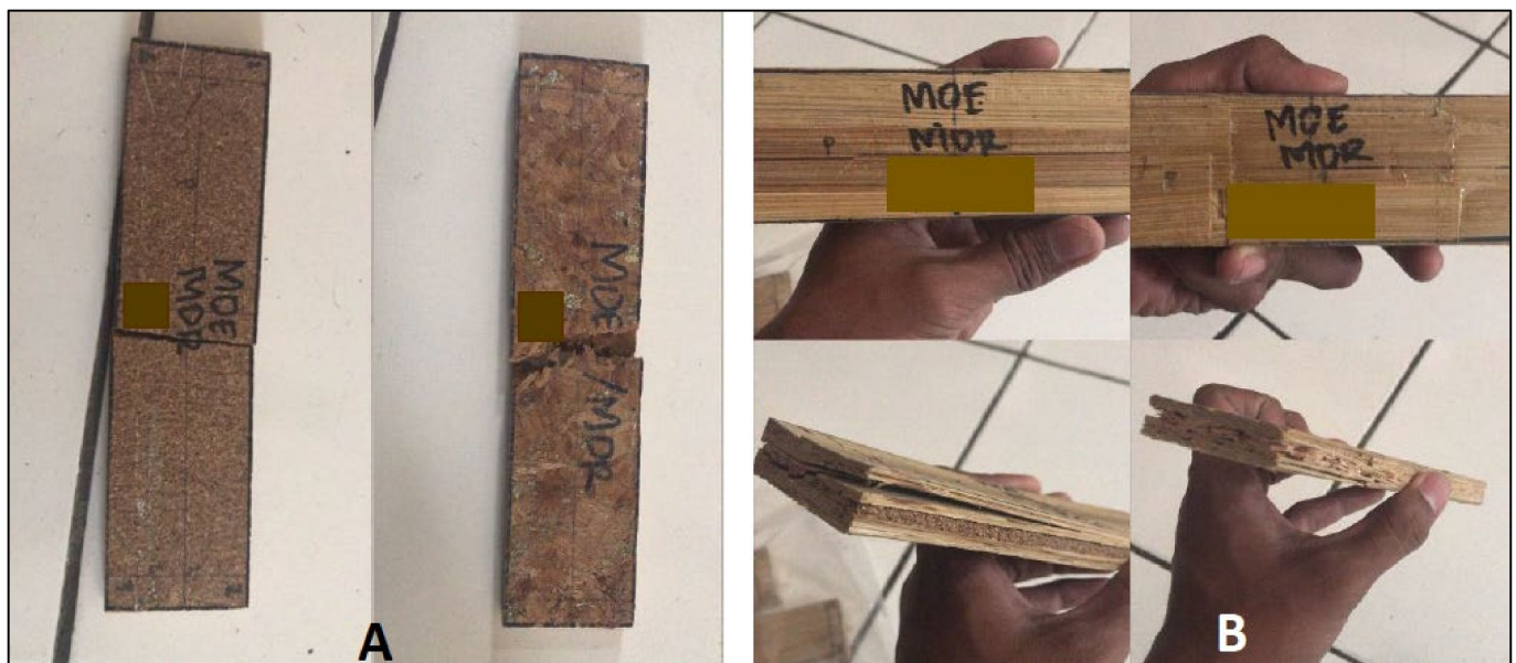
Figure 15. The appearance of damage in samples in MOE and MOR testing: nonstrand-coated board (A), and strand-coated board (B).
