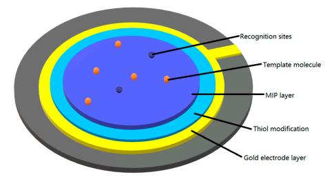
Figure 10. Schematic configuration of the QCM-MIP biosensor.
