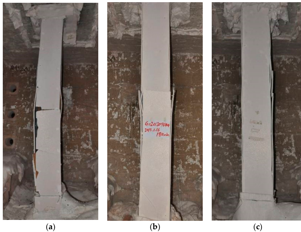
Figure 6. Columns after tests (still in the furnace): (a) HSS-C1; (b) HSS-C2; (c) HSS-C3.
