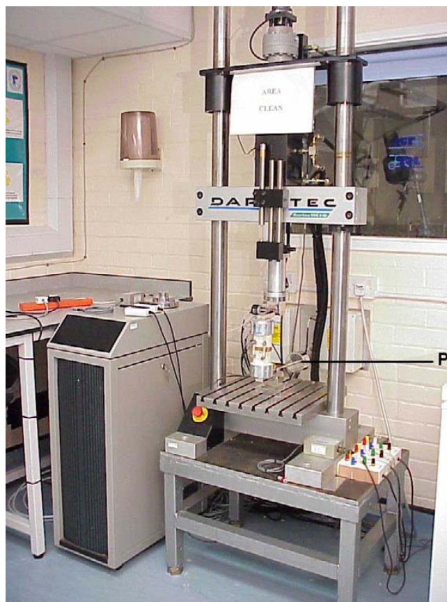
Figure 4 The Dartec® (Stourbridge, UK) material testing machine, with a spine model in the testing jig. A spine model is mounted in the jig, for eccentric loading using a 10 cm lever arm. 'P' indicates the position of the 50 N preload, applied through a 40 cm lever arm, in the opposite direction from the fulcrum, at the bottom end of the specimen.
