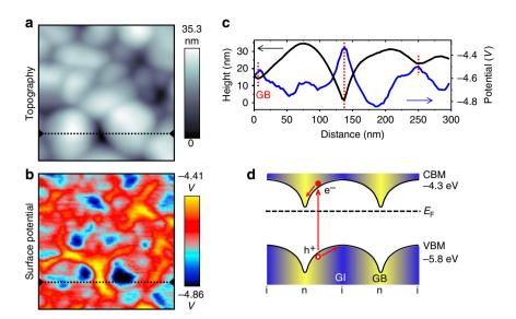
Figure 2 | Materials properties and device design. (a) KPFM topography and (b) surface potential image obtained simultaneously on one area. Image size for a and b:  $300 \times 300 \text{ nm}^2$  (c) Height and surface potential profile corresponding to the dashed lines in a and b. (d) Schematic of the band diagram in real space, illustrating how the photoexcited electrons slide down to the GBs while holes move towards GIs. i, intrinsic (blue regions); n, n-type (yellow regions).
