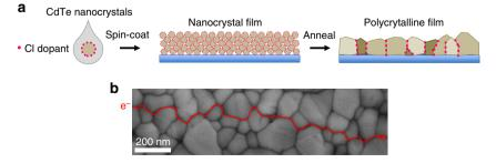
**Figure 1 | Materials design and fabrication. (a)** Schematic of the fabrication of a polycrystalline film from colloidal CdTe nanocrystals. Chloride-capped CdTe colloidal nanocrystals were spin coated onto a substrate forming a film, which was subsequently annealed at 350 °C in an argon environment for 0.5-5 min. (b) Scanning electron microscopy (SEM) image of the polycrystalline film. Red line and arrow represent a pathway along GBs for electron percolation.
