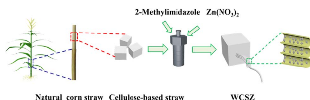
Fig. 1 Schematic of the fabrication of WCSZ composites.
