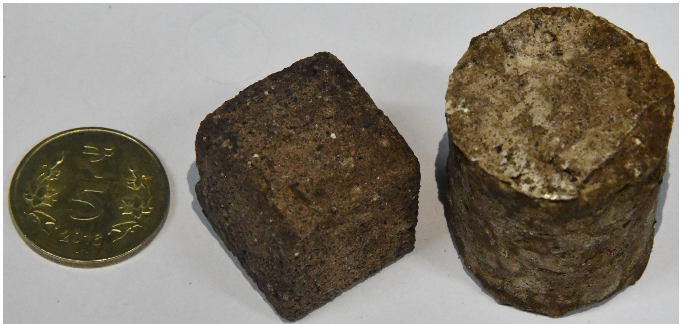
Fig 2. Representative image of consolidated samples using MSS. Such structures have been termed space bricks.
