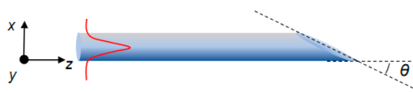
Figure 1. Schematic diagram of simulated subwavelength-diameter (SD) optical fibers with an oblique endface.
