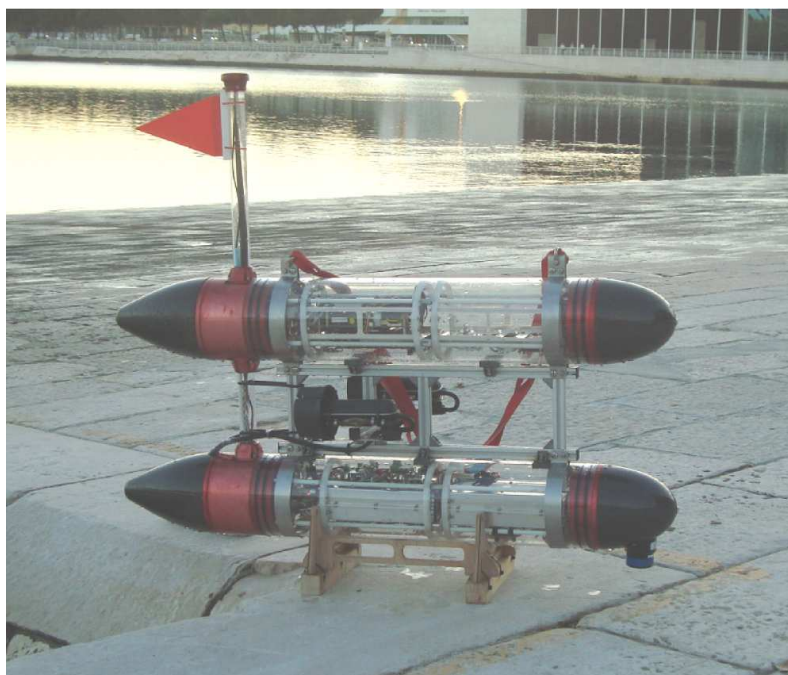
Figure 11. The Medusa autonomous surface vessel.
