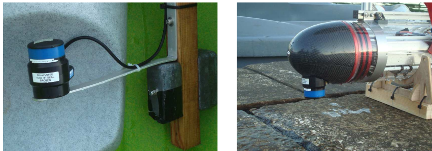
Figure 12. Fixed transponder (left) and acoustic modem/ranging device on the Medusa nose cone (right).
