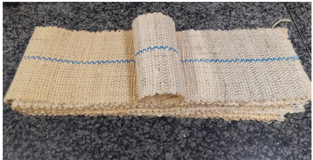
Figure 1. Fique fabric reinforcement.
