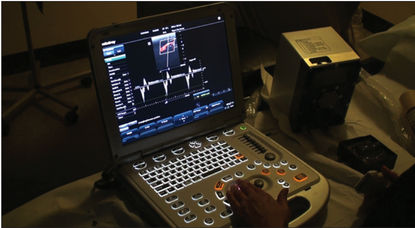
Figure 5 - Participant measuring simulated arterial stenosis. Duplex scanner is displaying both Colour and Spectral Doppler scan of stenosis being measured.
