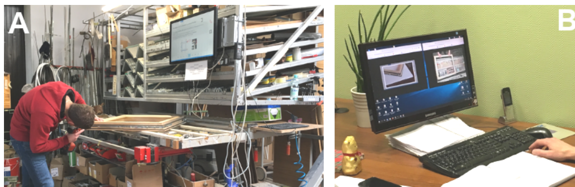
Figure 6. One of the testbed implementations for the proposed idea: (A) window assembly stand equipped with the speech- and touch-controlled HINT system, and (B) remote Avatar console.
