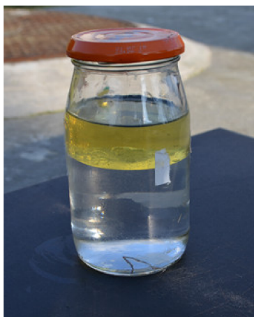
Figure 4. Condensate sample from landfill gas.
