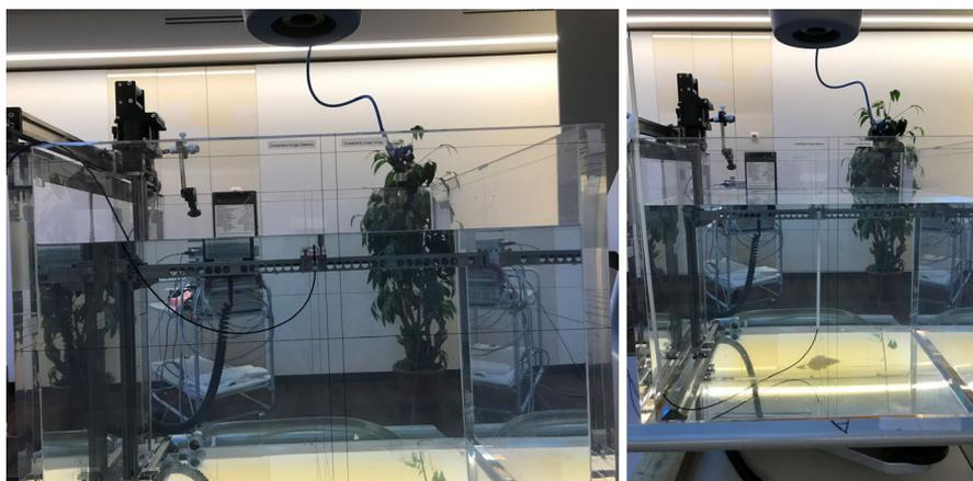
FIG. 1. Measurement setup to obtain the Cherenkov light ratio values. Left: minimum fiber configuration; right: maximum fiber configuration. [Color figure can be viewed at [wileyonlinelibrary.com](http://wileyonlinelibrary.com)]
