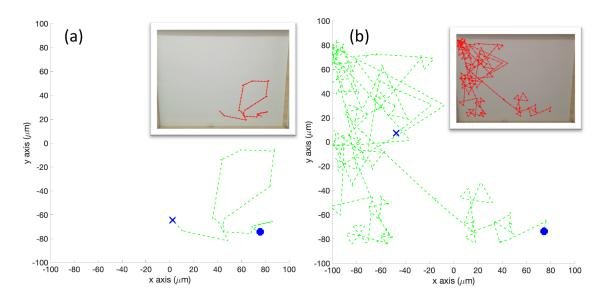
**Figure 13.** Case 4: Without obstacles, in the homogeneous/no effluent environment, typical trajectories of the e-puck robot running (**a**) the basic chemotaxis controller, and (**b**) the RapidCell chemotaxis controller. In each trajectory, the initial position is shown as a blue circle and the terminal position is shown as a blue "X". Positions corresponding to concentrations less than 1 mM are shown in dashed green, otherwise shown in red.
