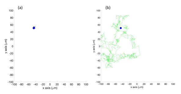
**Figure 16.** Case 7: With obstacles, in the homogeneous/no effluent environment, typical trajectories of the simulated robot running (**a**) the basic chemotaxis controller, and (**b**) the RapidCell chemotaxis controller. In each trajectory, the initial position is shown as a blue circle and the terminal position is shown as a blue "X". Positions corresponding to concentrations less than 1 mM are shown in dashed green, otherwise shown in red.
