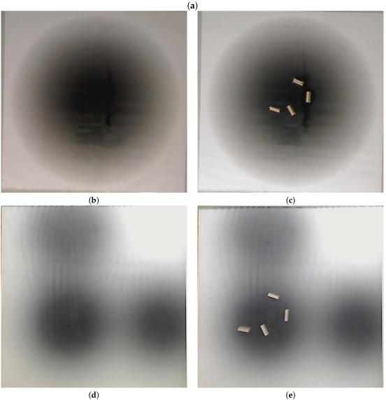
**Figure 4.** The e-puck robot used in the experiment can be seen in (a), with and without the "lid" used to make localization easier. The robots were tested on a grayscale gradient poster. Tests were done  $(\mathbf{b},\mathbf{d})$  without additional obstacles and  $(\mathbf{c},\mathbf{e})$  with obstacles in the middle of the poster. (**b**,**c**) represent the single-effluent environment while  $(\mathbf{d},\mathbf{e})$  represent the triple-effluent environment.
