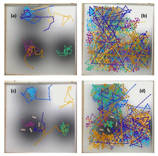
**Figure 23.** Summary of experimental runs with triple effluents for all seven initial positions that began on the area covered by the poster: (a) Basic controller, no obstacles; (b) RapidCell controller, no obstacles; (c) Basic controller, with obstacles; (d) RapidCell controller, with obstacles.
