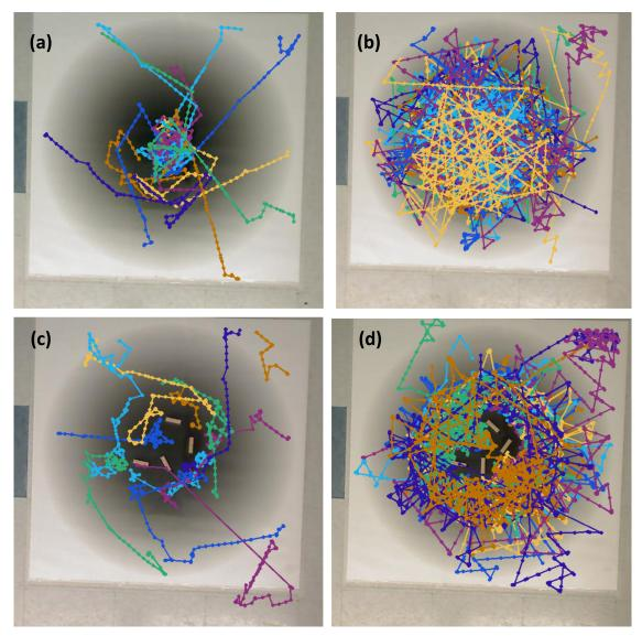
**Figure 22.** Summary of experimental runs with single effluent for all 12 initial positions that began on the area covered by the poster: (a) Basic controller, no obstacles; (b) RapidCell controller, no obstacles; (c) Basic controller, with obstacles; (d) RapidCell controller, with obstacles.
