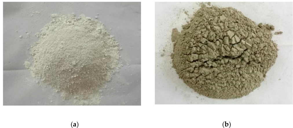
Figure 2. Macro morphology of mineral admixtures. (a) Metakaolin, (b) Superfine fly ash.
