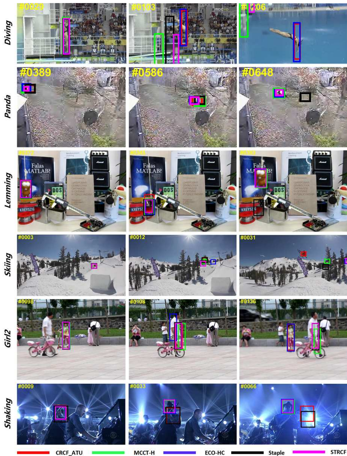
Figure 12. Tracking result visualization of our proposed CRCF_ATU tracker and comparative trackers on sequences Diving, Panda, Lemming, Skiing, Girl2, Shaking.
