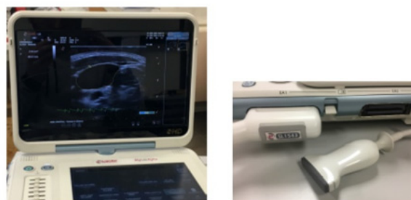
(a) My-LabAlpha system that displays the IJV contour (b) Linear array probe SL1543
