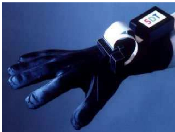
Figure 20. The 5DT Data Glove™ developed by Fifth Dimension Technologies; the glove measures seven DOF [74].
