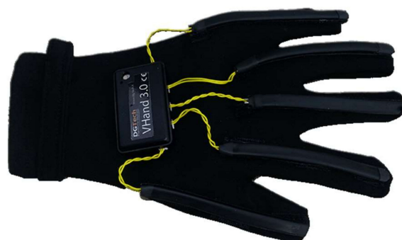
Figure 21. The A DG5-VHand glove equipped with five flex sensors and one 3-axis ACC [49].
