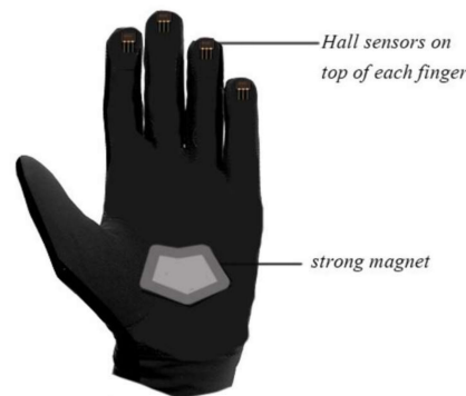
Figure 9. The sensory glove consists of Four Hall sensors on the tip of the four fingers [36].
