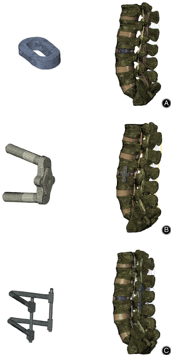
**Fig. 2** Finite element model with various fixation options. (A) Cage, stand-alone cage. (B) LP, cage with lateral plate and two lateral screws. (C) BPSR, cage with bilateral pedicle screws and rods.
