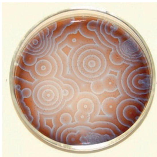
Figure 3. Patterns in the Belousov–Zhabotinsky reaction. Image courtesy of Michael C. Rogers and Stephen Morris, University of Toronto.
