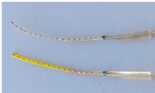
Figure 11. Representative image of uncoated (top) and hydrogel-coated (bottom) cochlear implant arrays. The coated array was soaked in a fluorescein solution for better visualization.
