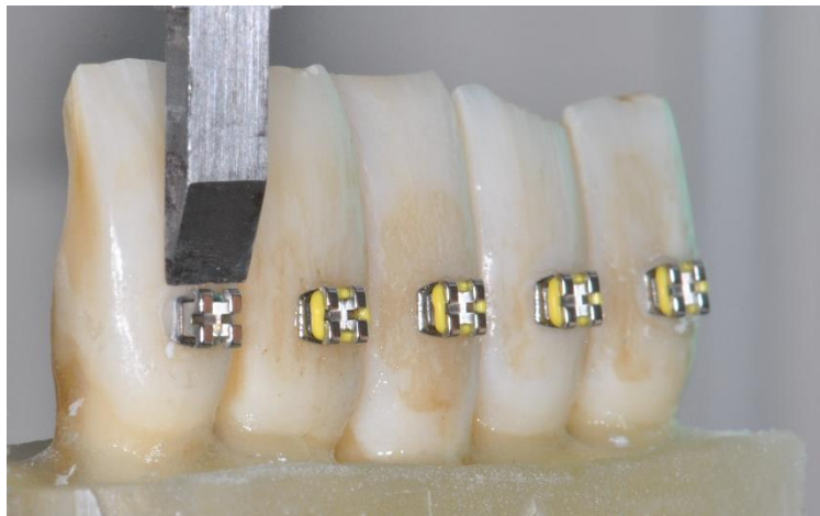
Figure 2. Shear bond strength test. The bracket base was set parallel to the shearing force.
