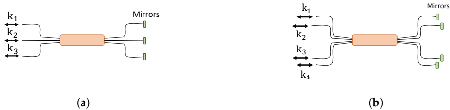
Figure 13. (a) Reversible integrated tritter. The photon propagation direction is reversed by placing mirrors at the end of the coupling region. (b) Reversible integrated quarter. It has the same configuration as (a) with an extra input and output port.
