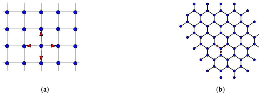
Figure 15. (a) Rectangular lattice. This structure has four edges for every vertex. (b) Hexagonal lattice. This structure has three edges for every vertex.
