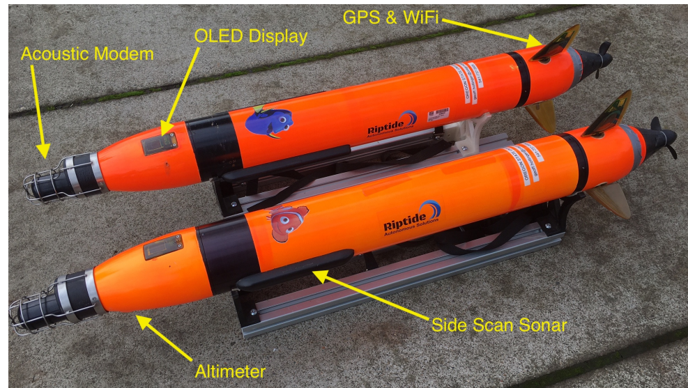
Figure 3. Riptide Autonomous Solutions micro-unmanned underwater vehicles (uUUVs) used for the experiments on Foster Reservoir, OR.
