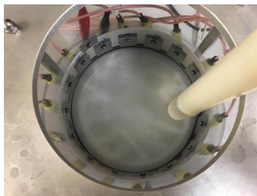
Figure 5. The experimental set up with the 2D ERT tank unit with tap water as a background.
